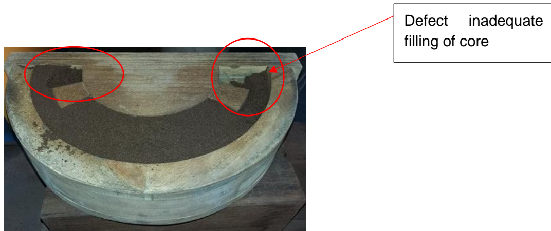
Figure 1: Core box traditional from traditional trial and error design with a defected core
